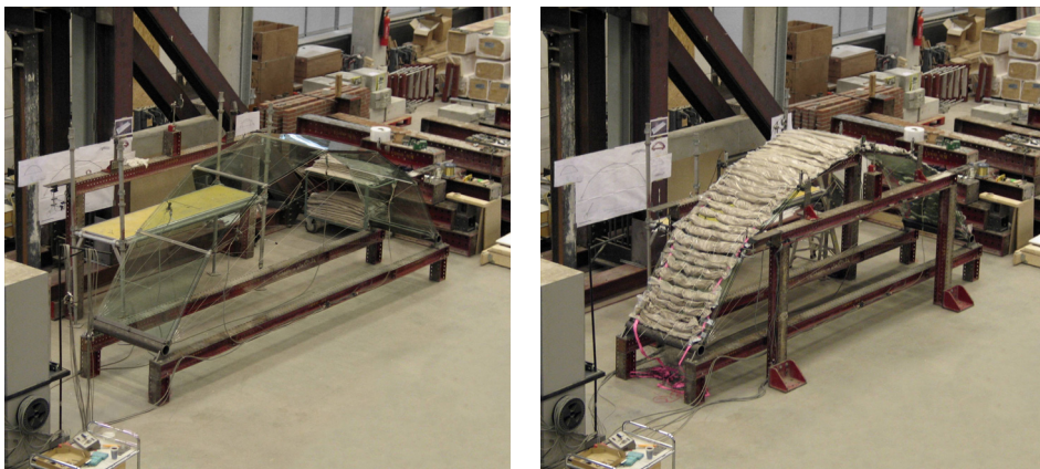
Figure 15ab: Test setup, before (left) and during (right) centric snow loading
