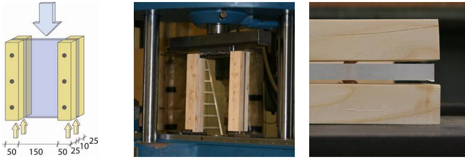
Figure 8a, b and c: Test setup with wood PMMA specimen.
