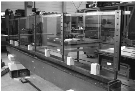
Figure 7: Specimen with temporary supports during curing of the epoxy adhesive.
