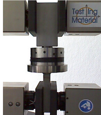
Figure 2: Photograph of point support specimen.
