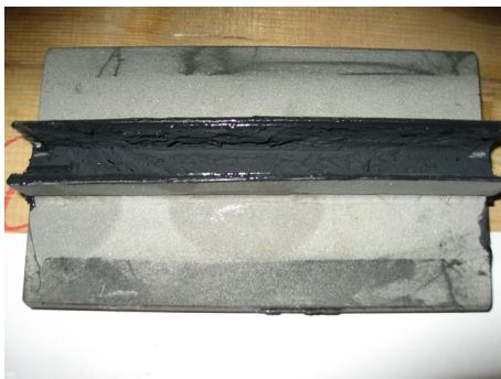
Figure 5a and b: Cohesive fracture pattern of a U-bonded specimen with a two-component silicone (left, K07) and of a channel-bonded one with a two-component polyurethane (right, K05)
