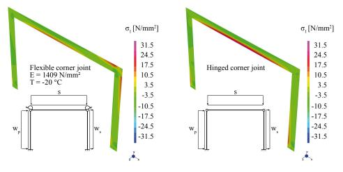
Figure 3: Stress distribution for different states of the structural system.
