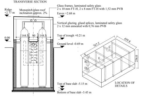
Figure 1: Fully glazed enclosure, transverse section (architects: Blum und Schultze Architekten, Dresden).
