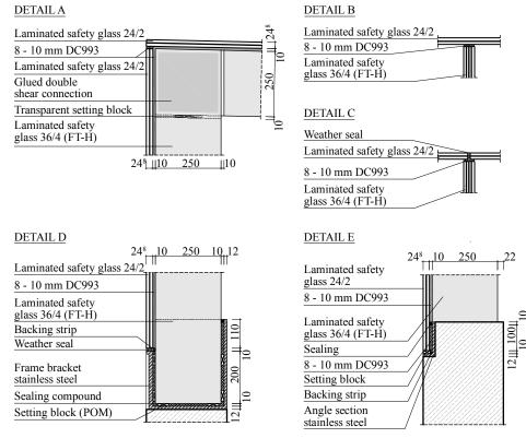
Figure 2: Details - frame corner (A), connection of vertical glazing and frame (B), connection of horizontal glazing and frame (C), base mount (D), connection of vertical glazing and concrete trough (E).
