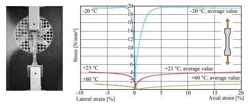
Figure 4: Tensile test for determining the material parameters, test set-up and stress-strain-diagram.
