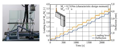
Figure 5: Verification of load bearing capacity: test set-up and results.
