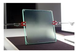
Figure 6: Studies of curing parameters - haze of the adhesive after curing with intense radiation power.
