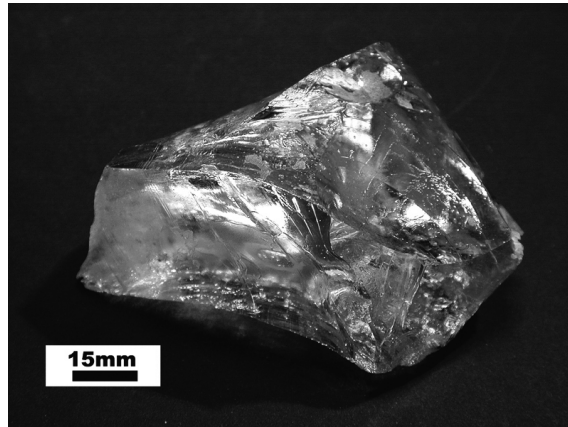
Figure 7: Part of a Roman glass ingot from les Embiez shipwreck, Côte d'Azur, still very fresh after 18 centuries spent in sea water [8]. This glass was likely made near Alexandria where the existence of natural ores of sodium carbonate gave a definite competitive advantage to local glass makers [9]. These exported ingots as well as finished products throughout the whole Mediterranean area, and even in Western Europe, where glass was extensively recycled, remelted and blown again, but not produced from raw materials before the third part of the first millennium [10].
