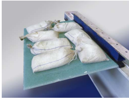
Fig. 3 Demonstration of the residual load-bearing capacity of laminated safety glass with structural PVB interlayer after breakage of both panes and planar load (Singh and Stelzer 2015).
