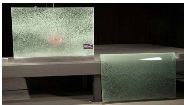
Fig. 1: Comparison of Structural Interlayer vs Standard PVB after Breakage (2 x 6 mm fully tempered and 1.52 mm interlayer)
