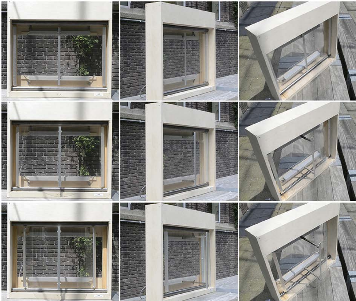
Fig. 14 Physical model developed with a 2mm thick thin glass panel and chain drive actuators
