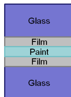
Fig. 8 Paint between two layers of film
