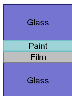
Fig. 7 Paint directly applied on glass
