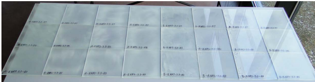
Fig. 9 Samples for the durability test with sprayed paint
