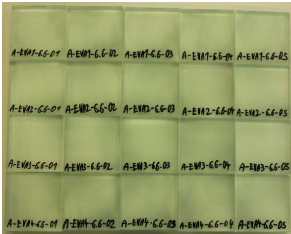
Fig. 11 Samples for the shear test with sprayed paint
