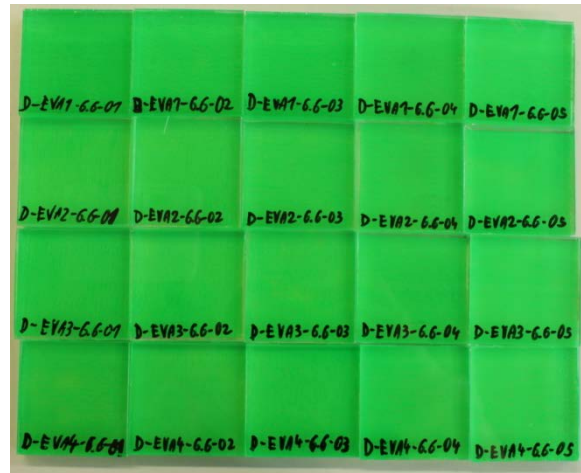
Fig. 12 Samples for the shear test with brush applied paint
