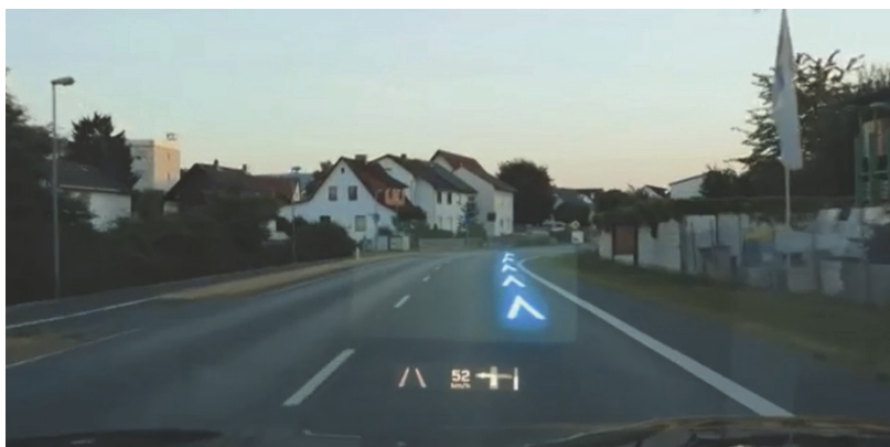
Fig. 3 Continental Augmented Reality Head-up Prototype: Augmented guidance and AR head-up display area (above) in combination with conventional head-up (below). In both cases the display area is visible as enlightened background in this image. Screenshot from (Continental/SAE 2018); 0:42 min. Image courtesy of Continental AG.
