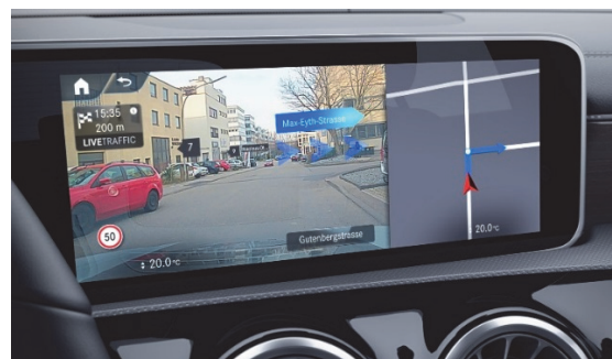
Fig. 1 A text message displayed in a huge head-up display which is not registered in three dimensions (left). Augmented video navigation display with guidance arrows registered at a fixed world position (right). Images courtesy of Daimler AG.
