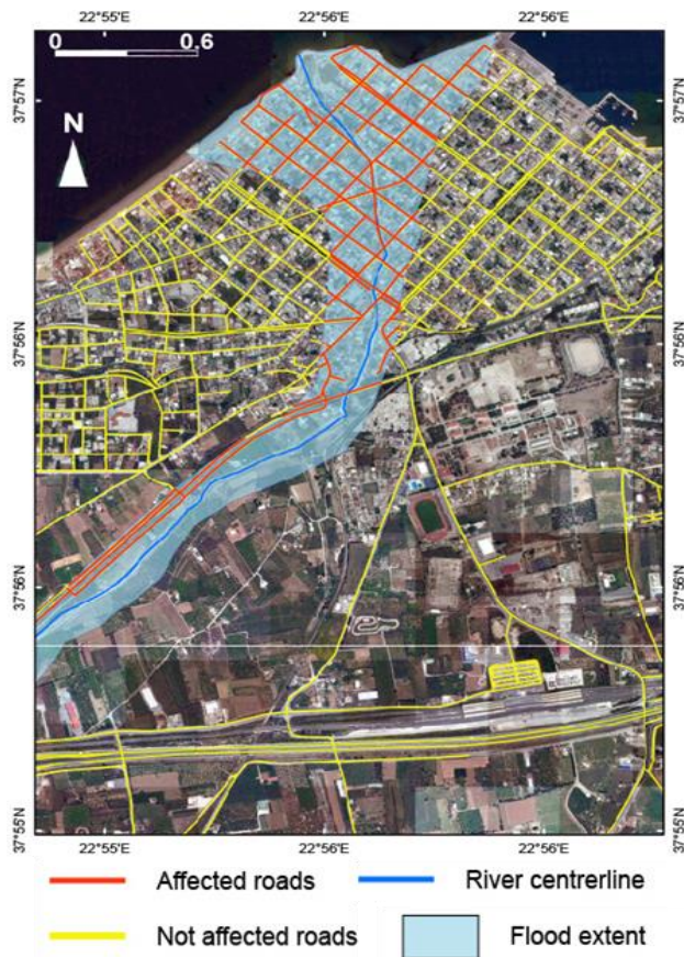
Figure 3. Maps of Xerias river basin near its outlet at the town of Corinth, illustrating the extent of flooding as mapped during the post-flood fieldwork, and the affected part of the road network
