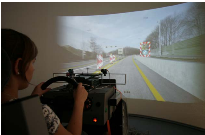
Figure 3. Traffic Sign Simulator mock-up with eye tracking system
