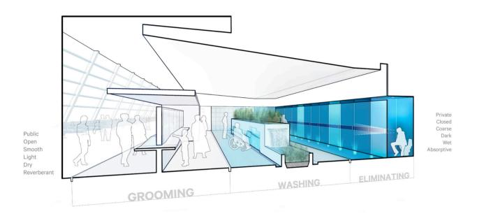
Section: As users circulate from one station to the next, passing from the outermost grooming station to the innermost toilet wall, they experience a multi-sensory gradient that takes them from public to private, open to closed, smooth to course, dry to wet, acoustically reverberant to sound absorptive, ambient to spot lighting.
