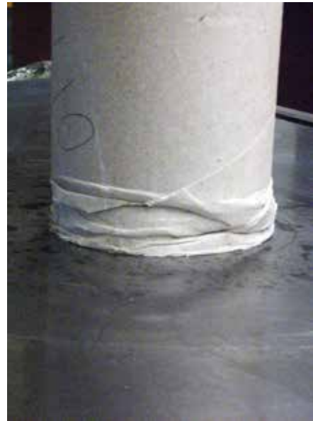
FIGURE 2.40 Paper tubes test on axial compression at TU Delft, wrinkles caused by axial compression
