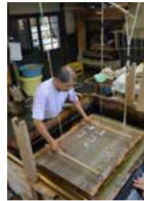
FIGURE 2.11 waving the screen previously dipped in the solution ( tame-zuki technique)
