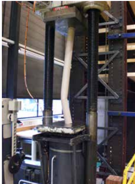
FIGURE 2.39 Paper tubes test on axial compression at TU Delft, noticeable buckling
