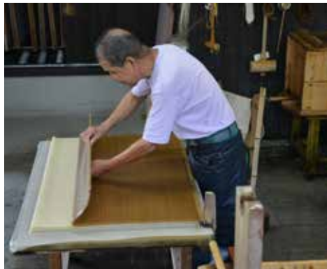
FIGURE 2.13 Placing the Washi paper sheets on the stock
