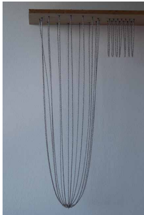
FIGURE 6.27 Catenary model of the initial design.
