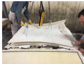
FIGURE 6.19 Demoulding of the free-form prototype.
