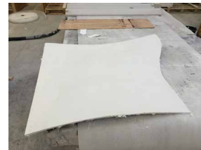
FIGURE 6.20 The finished free-form GFRC panel after demoulding.
