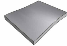
FIGURE 5.13 Finished free-form GFRC panel with an edge-return.
