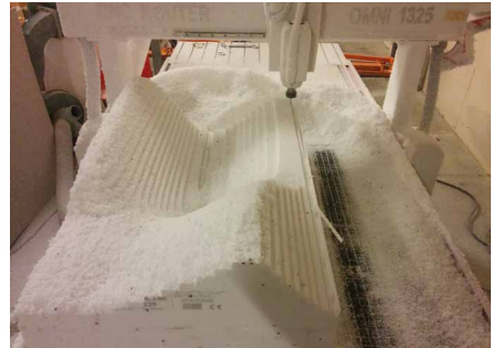
FIGURE 4.8 Concrete mould milled by a CNC machine
