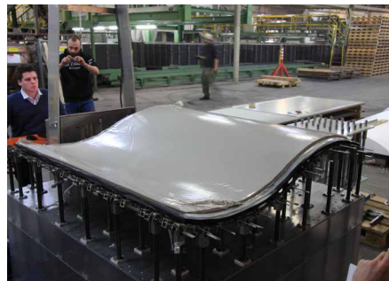
FIGURE 4.10 Automated premixed concrete panel placed on the digital flexible table in a single curved profile while curing
