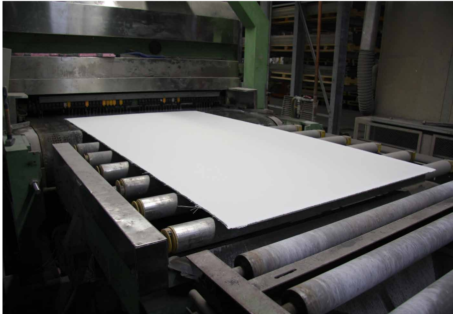
FIGURE 2.3 Automated process for flat thin-walled GFRC.
