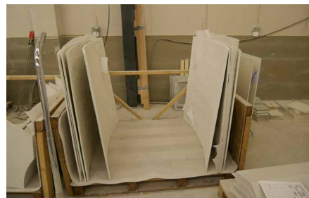
FIGURE 6.31 Finished cast panels for ring 1 and ring 2.
