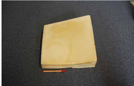
FIGURE 6.4 First sample of intermediate mould made with LDPU, (40cm x 40cm).
