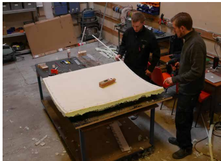
FIGURE 6.23 Plastic edge-barrier being fitted to the intermediate mould.
