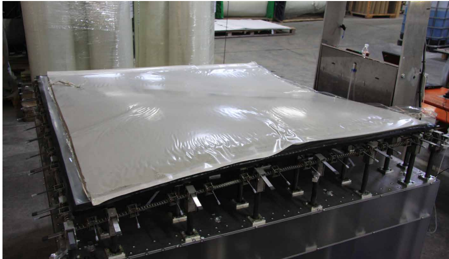
FIGURE 3.9 Testing of a thin-walled GFRC panel produced with the automated premixed process on a flexible table. The flexible table is positioned in a free-form shape
