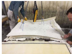
FIGURE 6.19 Demoulding of the free-form prototype.
