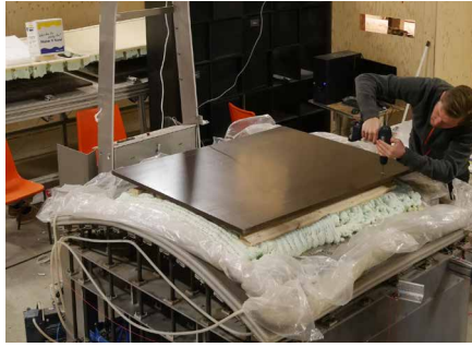
FIGURE 6.21 The simplified timber base plate being fitted to the foam part of the intermediate mould.
