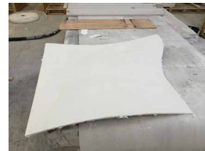
FIGURE 6.20 The finished free-form GFRC panel after demoulding.
