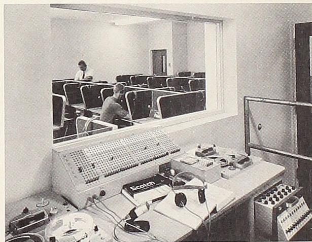
The Language Lab on the second floor offers 70 students the opportunity to listen to or speak in four languages simultaneously without being disturbed by each other. A professor using the monitor in the foreground can tune in on any one of these students at any time to praise or correct him.
