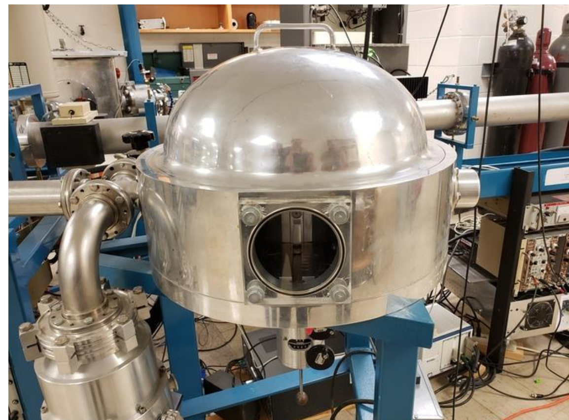
Fig 5. The chamber at the end of the line on the pelletron will scatter the proton beam to deliver radiation to the mice.
