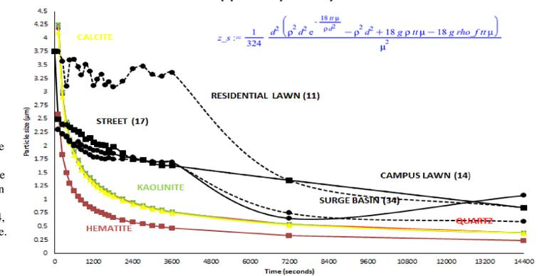
**Figure 7.** This graph shows the measured average particle size versus settling time from the FlowCam and DLS data (point to the white curves from each well) compared to a version of the Navier-Stokes equation with a term added to account for the non-spherical shape of the grains. Calcite, quartz, kaolinite, and hematite are shown here in comparison to the non-homogenous wells. Focus wells 11, 14, 17, and 34 are shown here.
