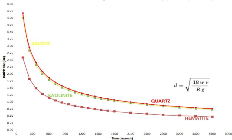
**Figure 2.** A relatively quick way of estimating particle size in the suspensions was to apply the Modified Navier-Stokes Equation to common natural mineral particles. The density of the non-iron particles is similar enough to have very little effect on settling time. These preliminary calculations were for sphere particles, which suggests that settling differences are driven more by particle shape than density.
