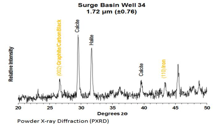
**Figure 6.** Measurements collected using PXRD show that both graphitized carbon black or graphite, reflector at 002, and iron, reflector at 110, appeared in the surge basin (34). The halite that appears in this sample is thought to be from the drying process in which the salt crystals would have been able to form.
