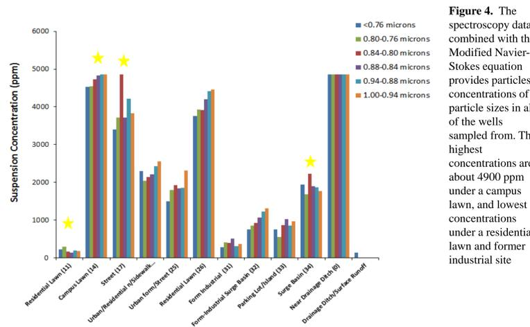
**Figure 4.** The spectroscopy data combined with the Modified Navier-Stokes equation provides particles concentrations of particle sizes in all of the wells sampled from. The highest concentrations are about 4900 ppm under a campus lawn, and lowest concentrations under a residential lawn and former industrial site
