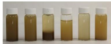
**Figure 1.** This is a demonstration of variation in well settling between well sampling localities and suspended sediment composition. Some photography was used to capture the shift in water clarity as the particles settled out of suspension during a 60 minute period. Notes that what is in suspension in the samples may or may not be reflective of what particles are suspended within the well due to the potential for disruption when samples are collected.
