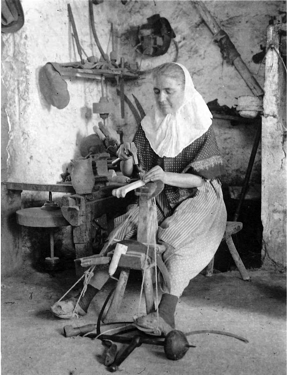
Fig. 6.—A woman making the teeth on a sickle blade by striking the blade with a hammer and chisel. After Llompart et al. , 1990:175.
