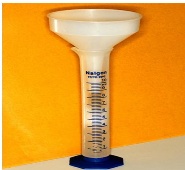
Figure 1 | A funnel was inserted into a graduated lab cylinder to collect saliva by volume
