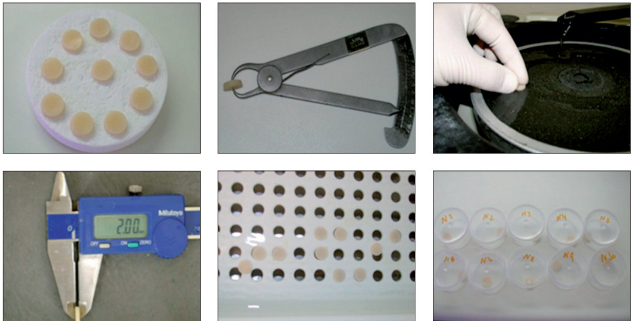
Figure 2 | Procedures to obtain a 2 mm sample free of dust.
