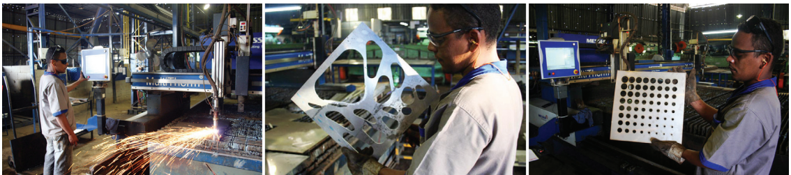
Figure 19. CNC plasma cutting process showing different designs.
