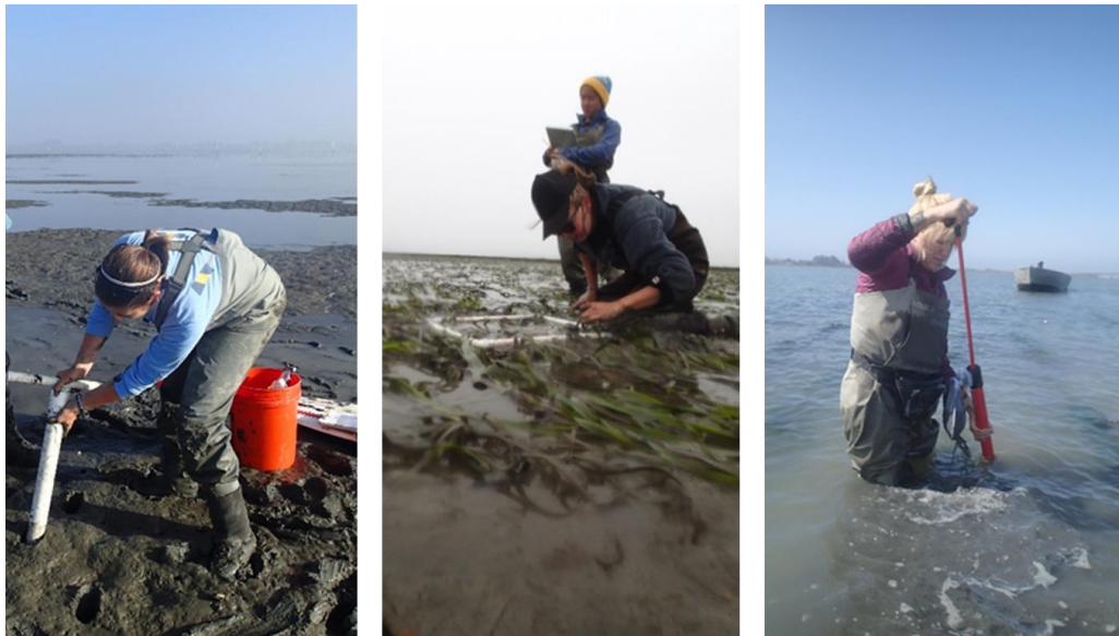
Figure 3. Left: Collection of 10cm deep sediment cores for benthic invertebrates and analysis for sediment characteristics. Center: Measuring eelgrass percent cover and shoot count using five 0.5m 2 quadrats along a 50m transect. Right: Collection of epibenthic organisms using a manual bilge pump with a 500micron net attachment.
