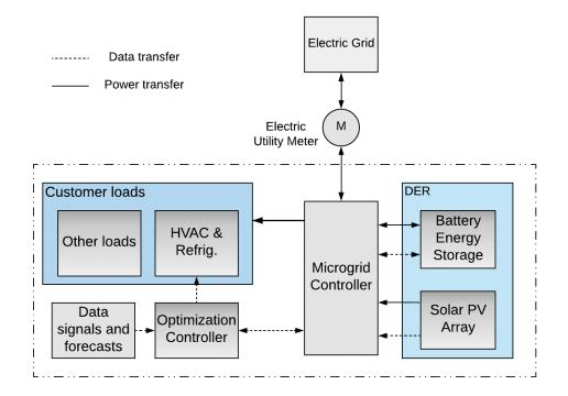
Figure 2. Example of basic MG with solar energy generation, and battery storage as the distributed energy resources, and a MG controller to manage all loads (grid, solar, battery, and customer).
