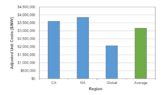
Figure 4. Regional average unit cost for MGs. Costs are based on the total cost over the sum of power capacity of all generation sources. Source: (Asmus et al. 2018).
