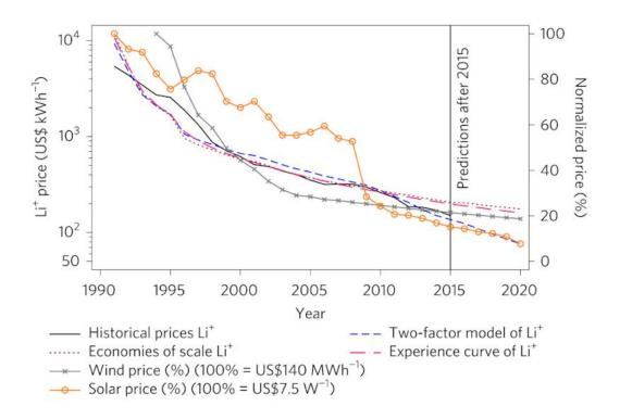
Figure 10. Comparison of traditional one-factor models for and the two-factor model to historical costs of lithium-ion. Wind and solar price reductions are normalized, see legend. Source: (Kittner et al. 2017).
