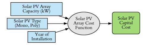
Figure 20. Solar PV Array Cost Function.
