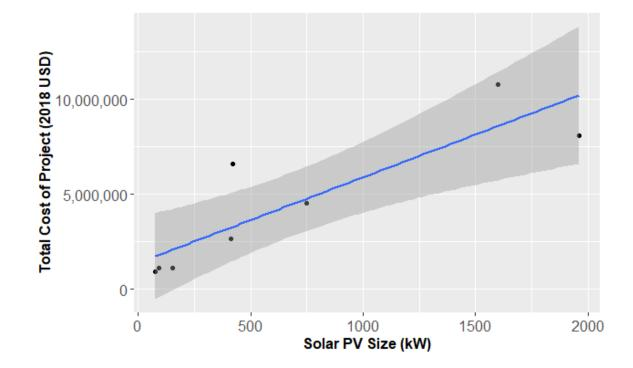
Figure 6. Total Costs of MGs According to Size of Solar PV Installed
