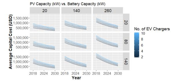
Figure 35. Estimated Total Cost for specified Solar+ Systems with Varied Component Sizes. This output is for a site with monocrystalline solar PV modules, and a battery system with a duration of 4 hours. Rows represent solar PV capacity and columns represent battery capacity.
