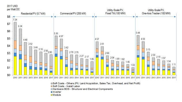
Figure 14. Benchmarked costs with cost breakdown noted for 2010 to 2017. Data is separated by system size and type. Source: (Fu et al. 2017).
