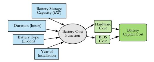
Figure 19. Battery Storage System Cost Function.
