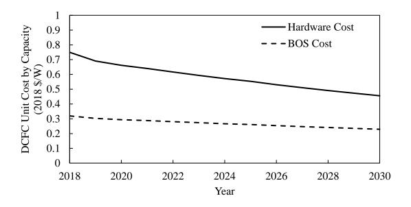
Figure 28. Cost projections for Direct Current Fast Charger Hardware and BOS cost from 2018 to 2030. Costs represent the installation of a single unit.
