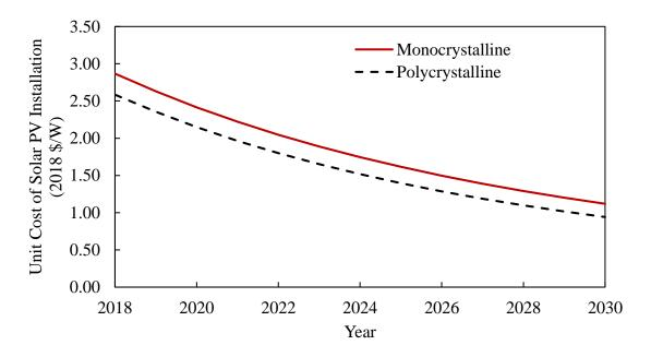
Figure 27. Cost projections for monocrystalline and polycrystalline PV array projects at 60 kW.
