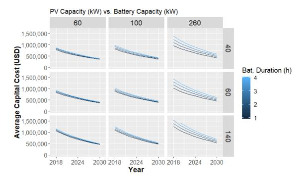
Figure 36. Estimated average cost for Solar+ systems with various battery and solar PV sizes. Plot is specific to a site with monocrystalline modules, and six EV chargers onsite. Rows represent solar PV capacity and columns represent battery capacity.
