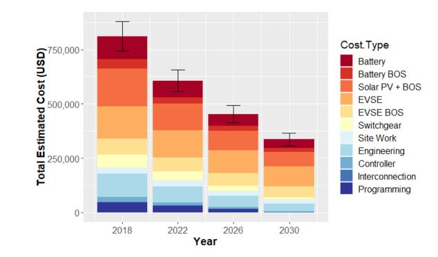
Figure 25. Expected cost breakdowns for a Solar+ MG constructed to serve a Medium C-Store. Error bars represent the 95<sup>th</sup> and 5<sup>th</sup> percentiles interval from all simulations from the Monte Carlo simulation.
