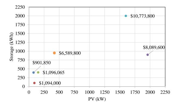
Figure 7. MG Case Study Capital costs depending on storage size (kWh) and solar PV size (kW).
