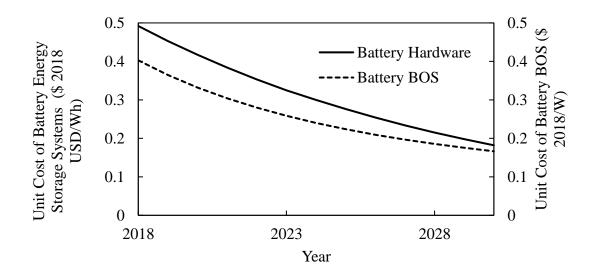
Figure 26. Average Cost Projections for Battery Hardware (\$/Wh) and BOS (\$/W). Note secondary axis reports the cost of BOS).
