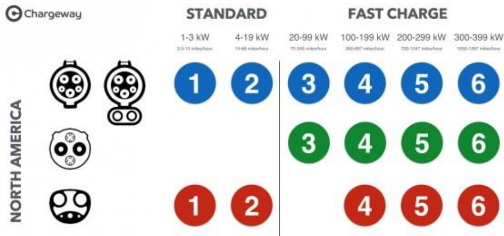
Figure 19: This image shows the proposed Chargeway design language, which codes according to color (charging standard) and number (charger power). (Chargeway, 2018)
