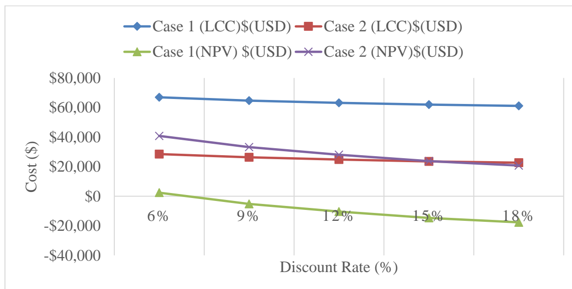
Figure 24. Sensitivity Analysis on the Life Cycle Cost and NPV as it Varies with Discount Rate for Case 1 (Self-Funded) and Case 2 (Grant Funded).
