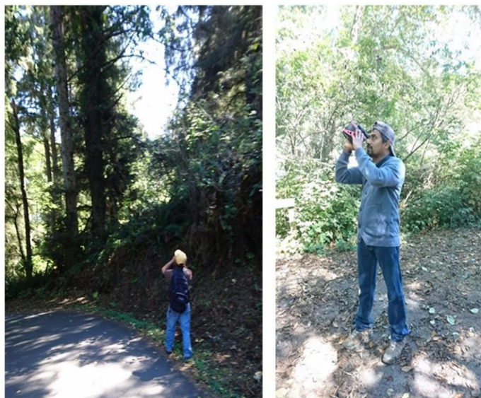
Figure 2. Measuring tree height using an Impulse Laser Rangefinder.
