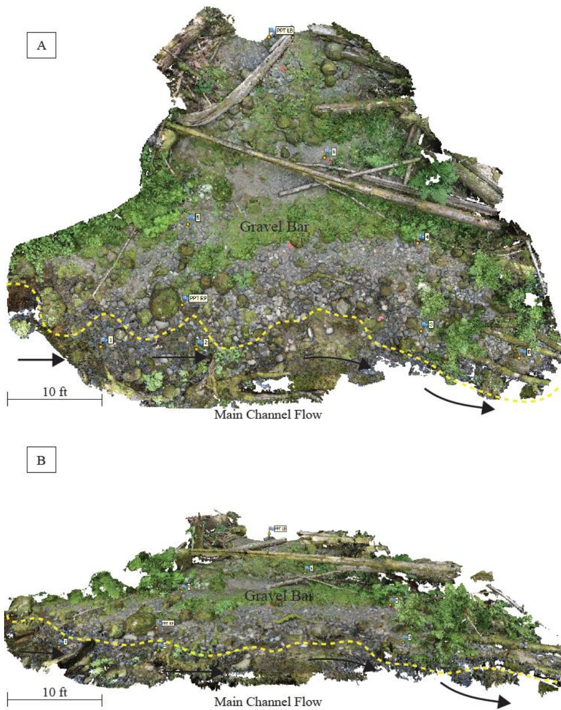
Figure 17. Dense clouds (not photographs) of Site 4: A) planview of Site 4 with GCPs and flow indicated, B) Oblique view of Site 4 with GCPs and flow indicated. Dashed line is approximate edge of water at 100 cfs.
