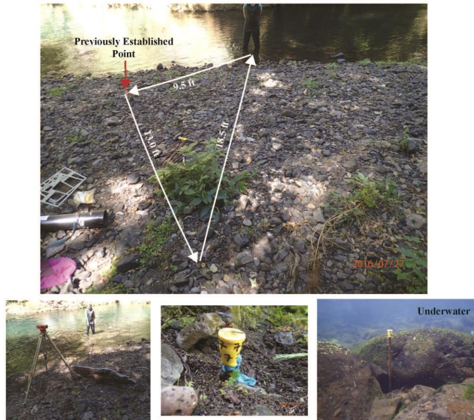
Figure 13. Photos of GCP setup and examples of GCPs above and below water.
