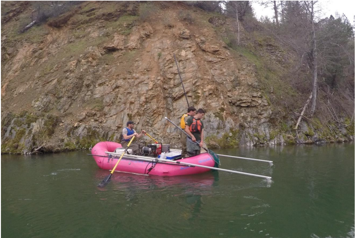
Figure 2. Electrofishing raft used to sample Brown Trout on the main stem Trinity River. Two netters stood in the front of the raft using nets with openings approximately 0.6m x0.3m and a handle between 1.75 and 3 meters long. Protruding in front of the netters were two 2.5 meter booms which held the anode fore on each side of the raft. The anode end consisted of four 1.5 meter wires that hung into the water. The silver tubes at the waterline under the oarlocks had 1.5 m cathode wires hanging down.
