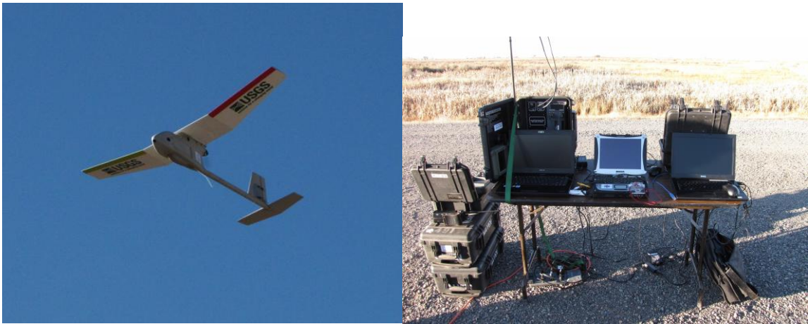
Figure 3. RQ-11A Raven UAS and ground control station (photos courtesy of USGS)
