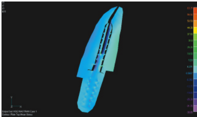
FIGURE 1 - Maximum tensile and compressive load stresses for the stainless steel Flexi Post.
