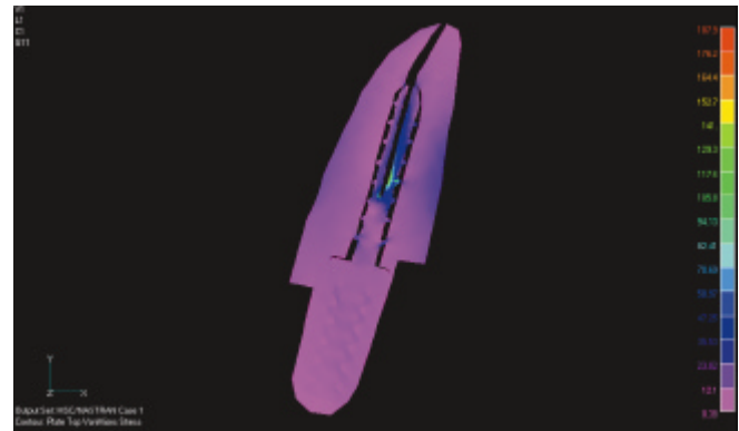
FIGURE 2 - von Mises stresses on the titanium Flexi Post.
