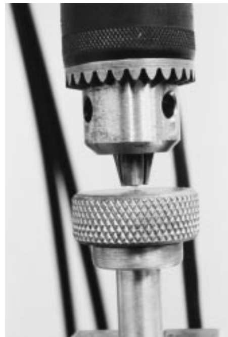
FIGURE 3 - Metallic frame containing a carbon fiber post positioned in a mandrel adapted to the Instron machine for tensile testing.
