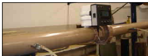
Figure 3 – Electronic Drag Force Flowmeter developed in this research installed on a pipeline.
