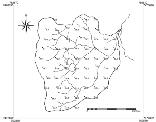
Figure 5 - Map with drainage and soil fine sand percentage point values (depth of 0 to 20 cm) in the studied watershed.
