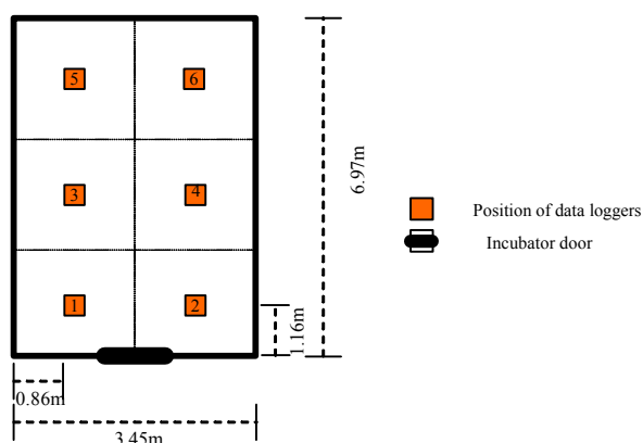
Figure 1 - Division of areas and data loggers' position inside the incubator where the samples were taken.
