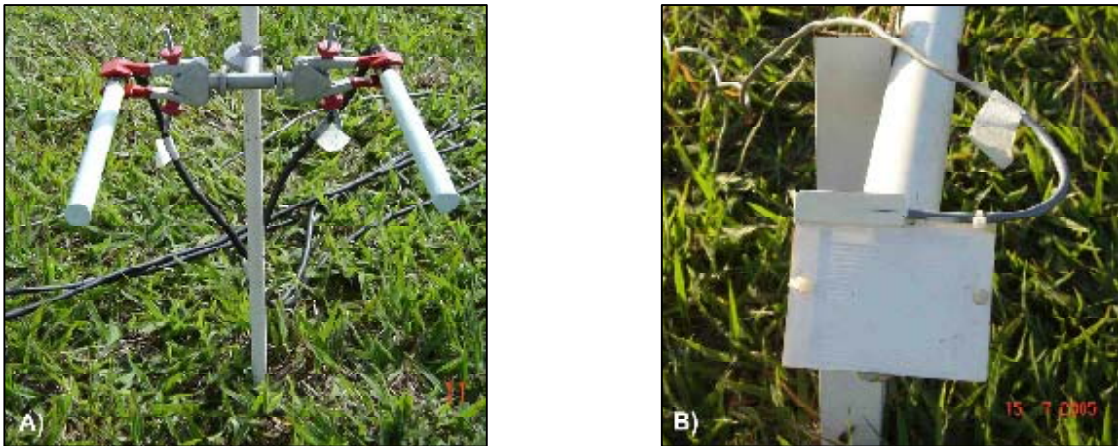
Figure 1 - Electronic leaf wetness duration (LWD) sensors: cylindrical (a) and flat plate (b).
