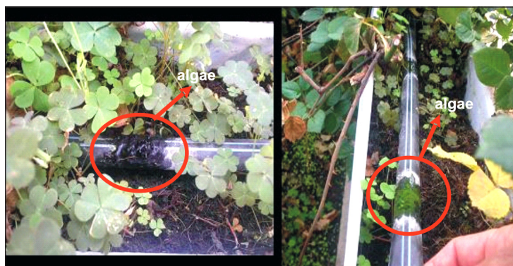
Figure 2 - Detail showing the formation of algae in the external part of the lateral lines of the evaluated sectors.
