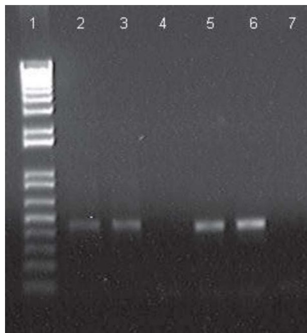
Fig. 1 - Ethidium bromide-stained agarose gel showing the products resulting from RT-PCR amplification performed with Alphavirus genus-specific primers, MAYV specific primers, RNA extracted from the patient (lanes 2 and 5) and MAYV positive control (lanes 3 and 6), respectively. Negative controls are shown in lanes 4 and 7 and molecular markers are shown in lane 1.
