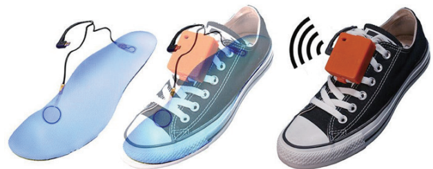
Fig. 2. Electroskip sensor positioning under toes and heel.
