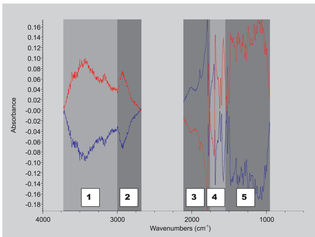
FIGURE 2 - Subtraction between the spectra of samples with high and low concentrations of amoxicillin in selected subregions.
