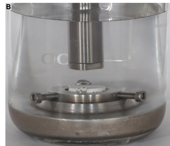
Figure 3- (A) Device used for centering the specimens. (B) Sample in deionized water for treatment with microtip. Centering of Y-TZP discs at the bottom of a beaker containing deionized water
