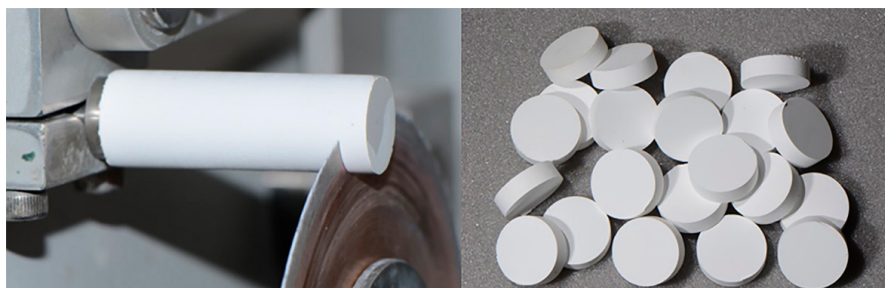
Figure 1- Preparation of specimens by turning and cutting pre-sintered ceramic blocks
