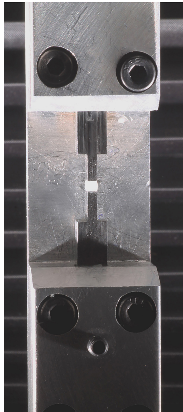
Figure 2- Universal Testing Machine (INSTRON) and metallic bases with composite specimen in position
