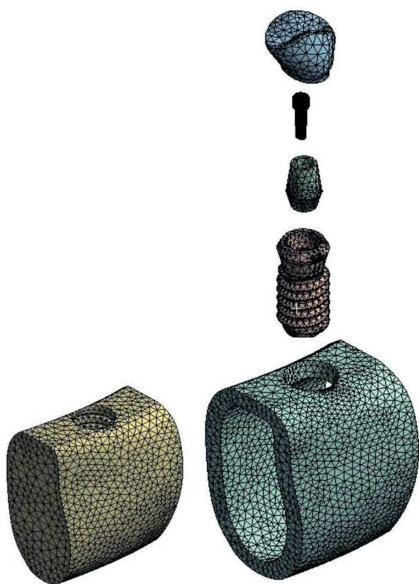
Figure 3- Bone-implant system mesh using tetrahedral quadratic elements
