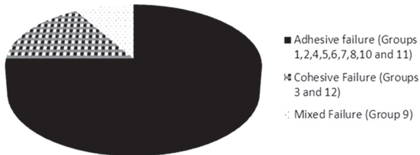
Figure 2: Type of bonding failure for all groups
